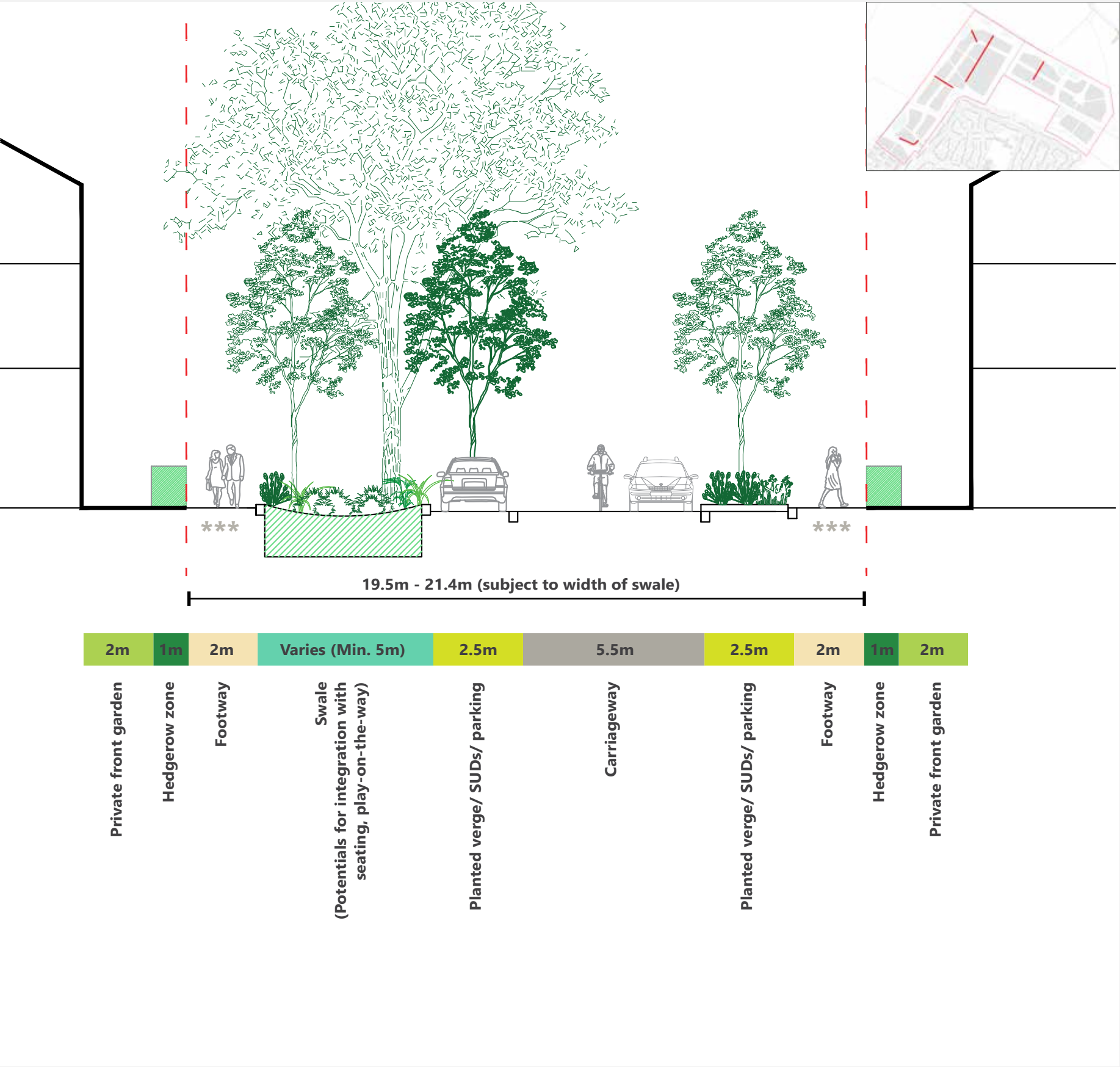
Fig. 6.27: Type 2B (swale on one side) - Typical illustrative section
