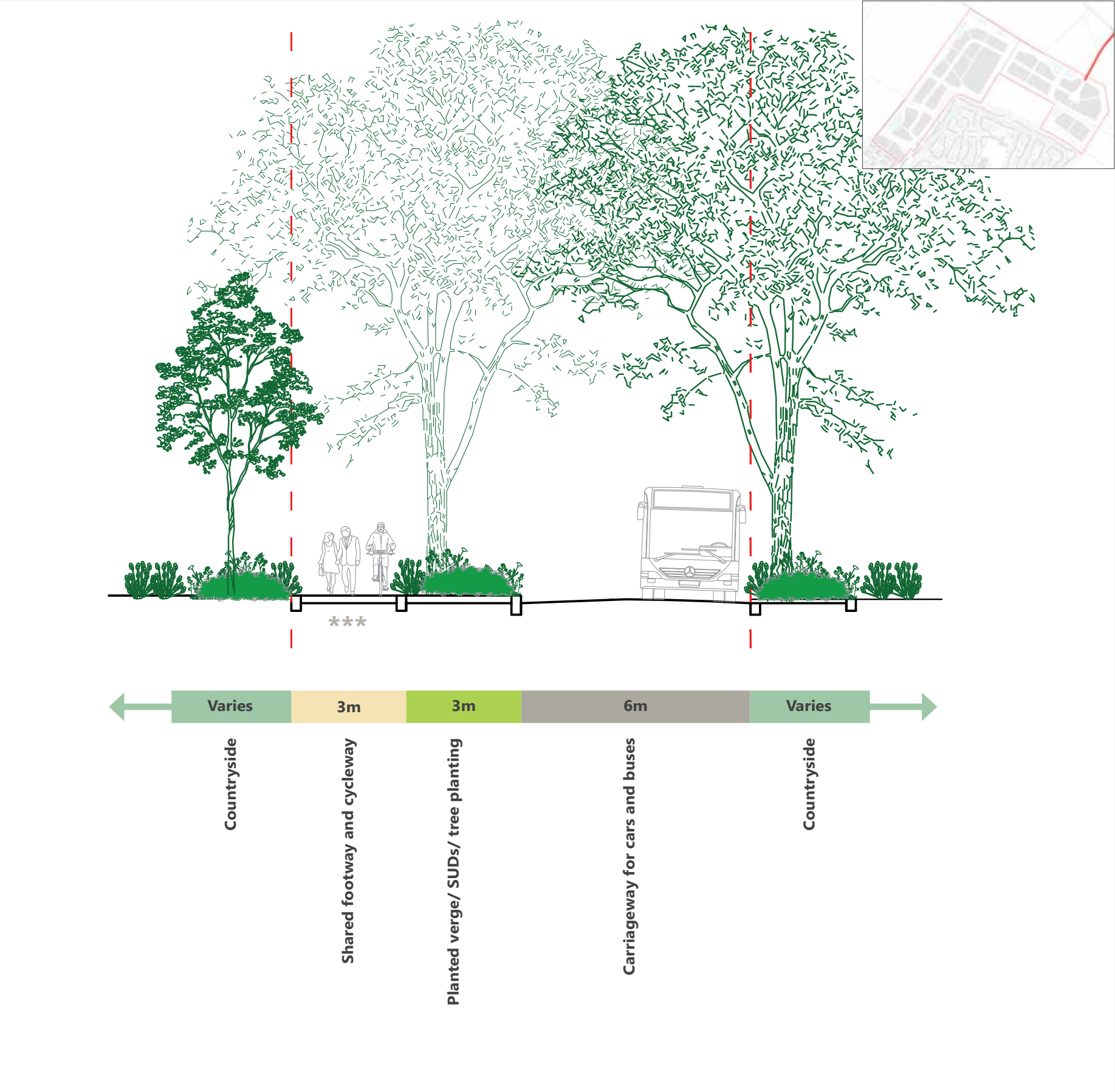
Fig. 6.44: Type 4 - Typical illustrative section
